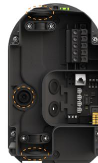
Pop out the pre-fitted rubber grommet at the selected AC supply cable entry point: top, rear **or** bottom. **Recommended entry options are shown later.**
