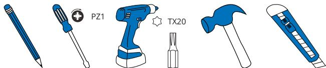
The following screwdriver heads are needed for installation:
