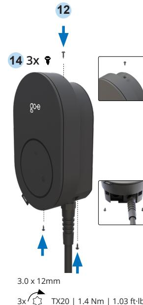
Secure the Charger in place using 3x TX20, length 12 mm screws and a Torx screwdriver, **applying a torque of 1.4Nm ± 0.1Nm**.
