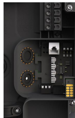
Pop out the small rubber grommet at the selected cable entry point: top or bottom.
